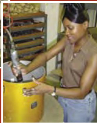
Each USA Custom drum is fitted with Gretsch's heavy die-cast lugs, and will later receive the manufacturer's signature die-cast hoops.
