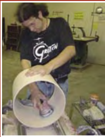
Gretsch USA Custom shells are carefully sanded inside and out.
