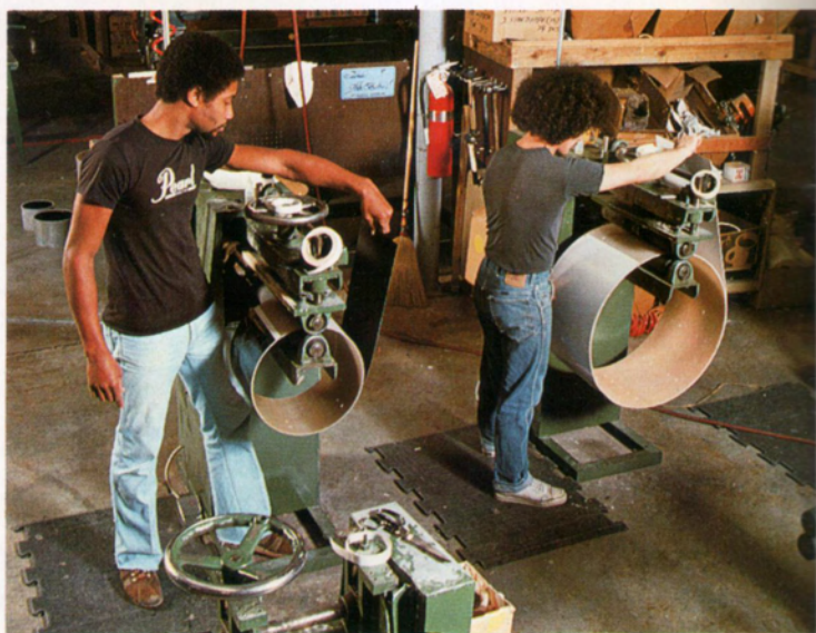
Applying covering material
