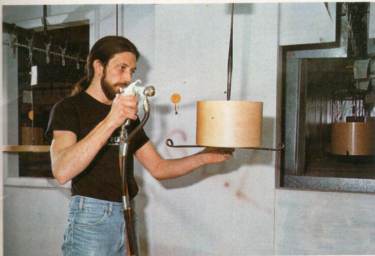
Spray booth with modern overhead conveyor system
