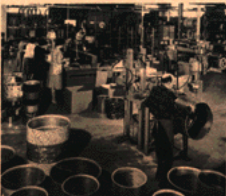
FINAL ASSEMBLY OF DRUMS
