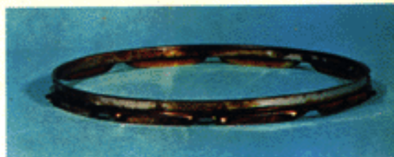
Chrome plated steel hoop, as used by our principal competitors and Japanese, after accelerated rust test.
