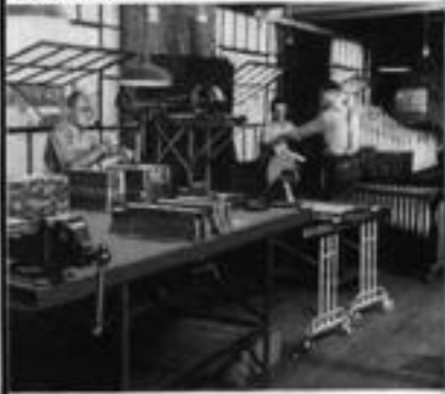
Here seasoned bars are tuned, drilled, stamped and strung for mounting on xylophone and marimba frames.
