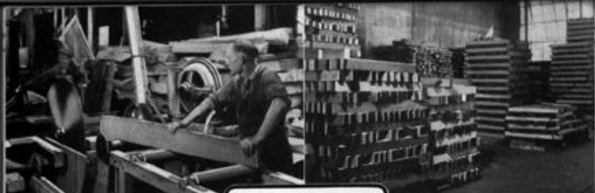
Slabs are cut into rough-bar stock and stored for further seasoning before cutting into xylophone and marimba bar sizes.
