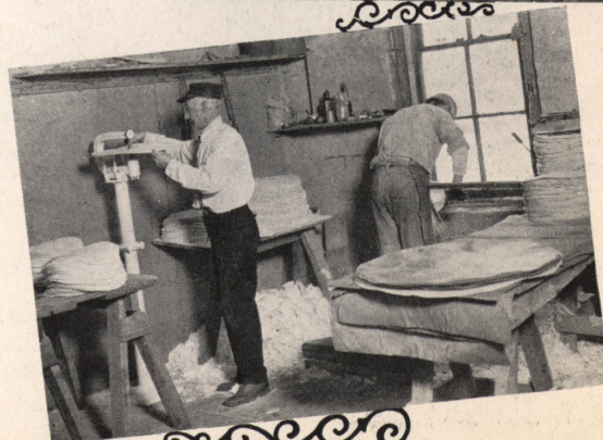
Gauge Inspection and Hand Shaving
