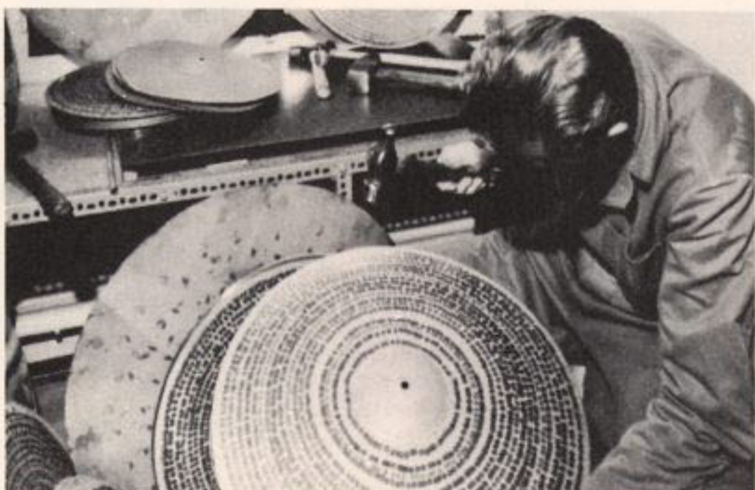
Careful hand-hammering of the PAISTE Formula 602 disc.
