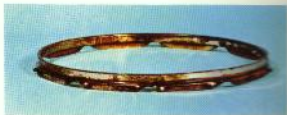
Chrome plated steel hoop, as used by others after accelerated rust test.
