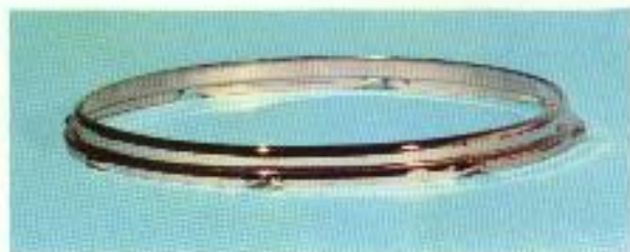
Slingerland chrome plated solid brass counterhoop after accelerated rust test.
