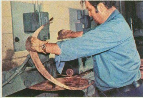
Blank is sheared to circular shape and center hole punched for lathing.
