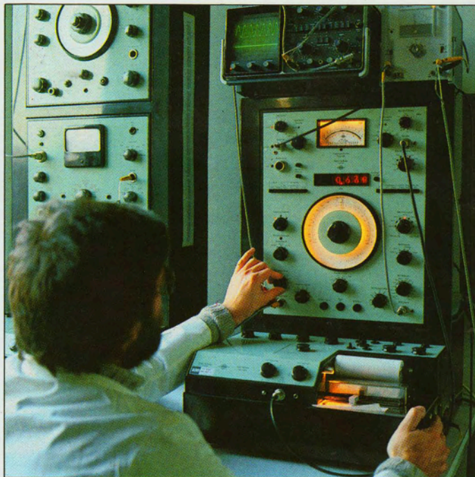
Scientific research on drums: Measuring with a Third Octave Analyzer and a Beat Frequency Oscillator
