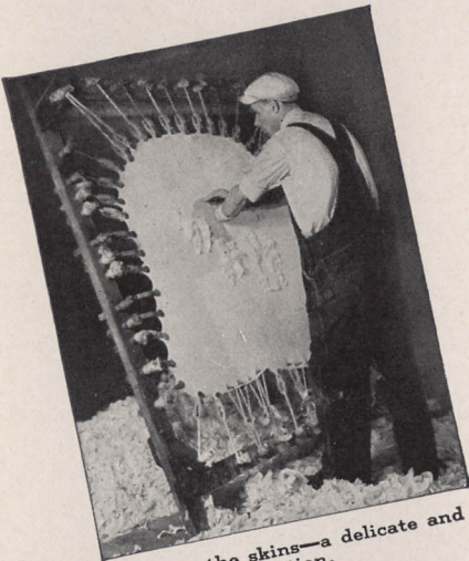
Stretching selected calfskins for Ludwig & Ludwig drum heads.
