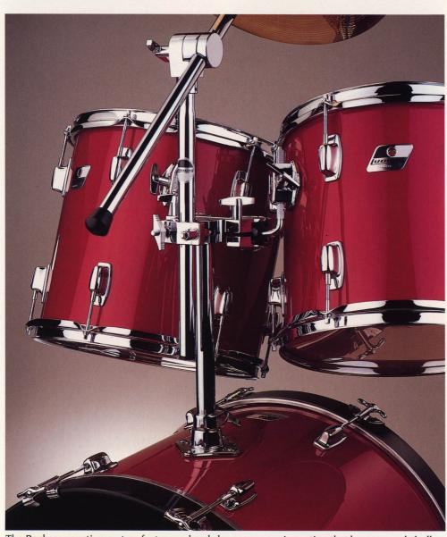
The Rocker mounting system features a hard chrome sure-grip casting that houses a poly-ball for full,  $360^{\circ}$  tom angle adjustment. The unique gate-style clamp lets you customize your kit with a variety of add-ons, including the LM-451-CH cymbal holder shown here. Ludwig Quik-Sets (standard with the system) add stability, speed set-up.
