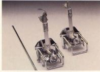
The famous P-70 Super-Sensitive strainer has a fast-action, double-end throw-off that keeps snares under consistent, even tension when released from the head. Dual tension adjustment accommodates both swivel and individually-adjustable parallel-action snares. Use with P-47 Super-Sensitive butt.
